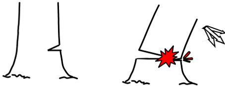
Opening too narrow - notch closes too early - hinge breaks: poor control
