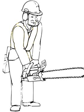
Figure 7: Starting saw off the ground
