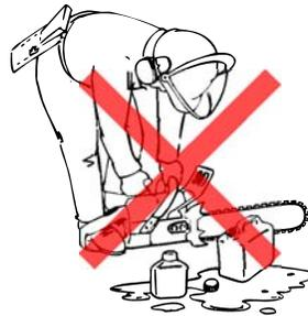
Figure 5: Do not start the saw at the place of refuelling
