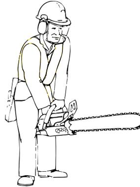
Figure 7: Starting saw off the ground
